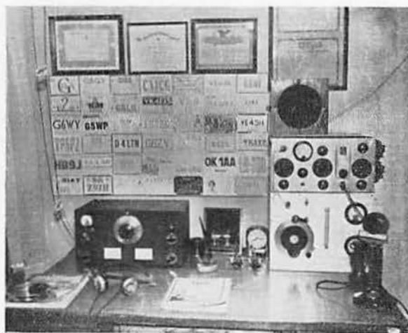
The operating end at W9NY. The cards confirm 28 Mc. contacts made during 1935. The receiver to the left is a National HRO. The transposed feeder goes to the send-receive switch. The remaining gear is concerned with police radio work.
